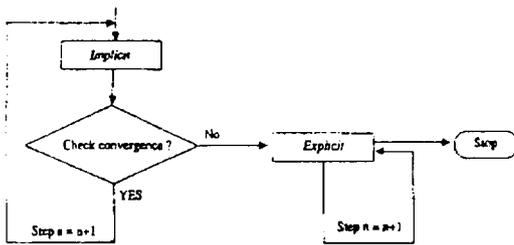
Fig. 1. Flow chart for the step-wise combined implicit-explicit scheme.
