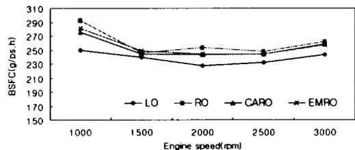
Fig. 4. BSFC vs. engine speed for each fuels at full load.
