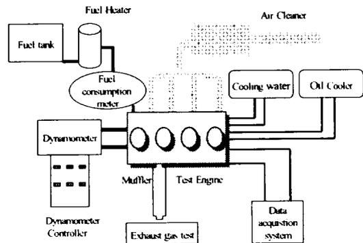
Fig. 1. Schematic diagram of the engine performance test system.
