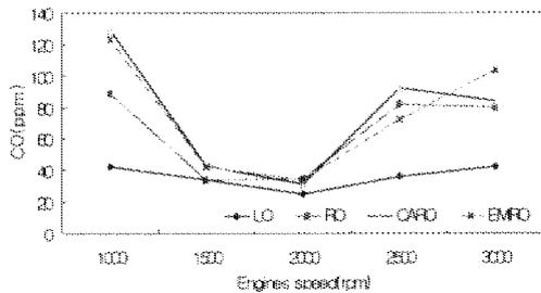
Fig. 5. CO vs. engine speed for each fuels at full load.
