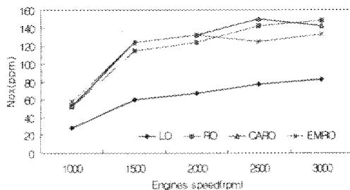
Fig. 6. NO<sub>x</sub> vs. engine speed for each fuels at full load.
