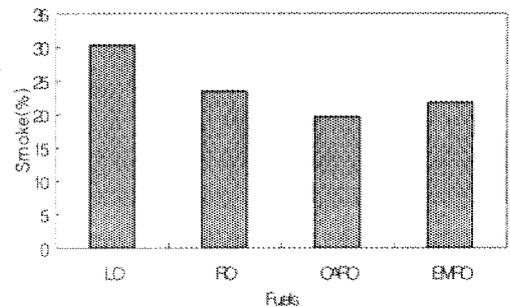
Fig. 7. Smoke emissions vs. engine speed for each fuels at quick acceleration.
