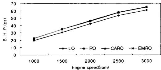
Fig. 3. Brake horse power vs. engine speed for each fuels at full load.
