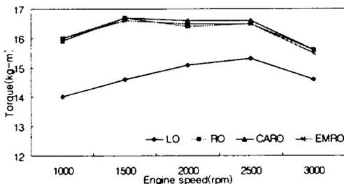
Fig. 2. Torque vs. engine speed for each fuels at full load.
