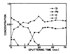
Fig. 5 AES depth profile of the Sample annealed at 900°C for 20s by RTA.
