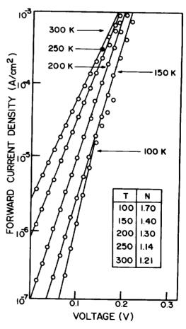
Fig. 7 Foward current density-voltage characteristics of Pd on n-type Si (100) as a function of measured temperatures.
