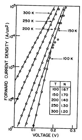
Fig. 6 Foward current density-voltage characteristics of Pd on n-type Si (111) as a function of measured temperatures.
