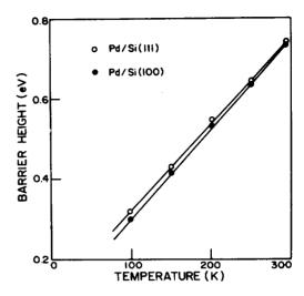
Fig. 9. Change of the barrier height of Pd on n-type Si(111) and Si(100) as a function of measurement temperature at 100 K to 300 K.
