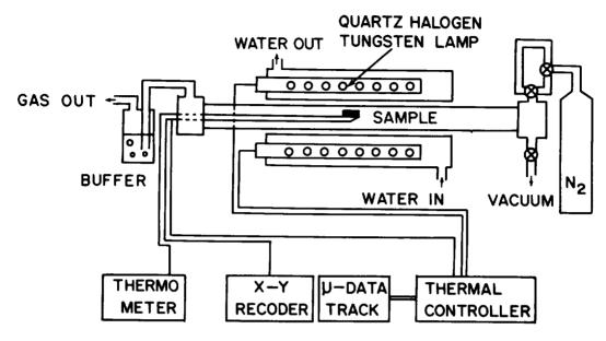
Fig. 1 Schematic diagram of a RTA System.
