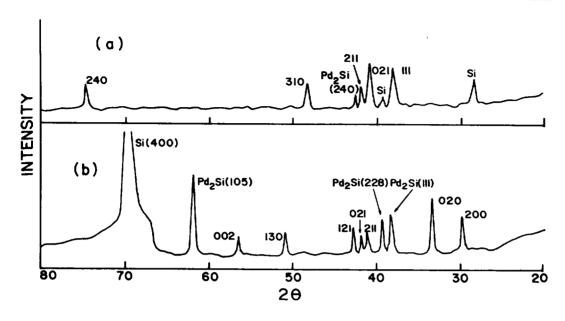
Fig. 3 X-ray diffraction spectra of the samples processed by the RTA at 900°C for 20s;
