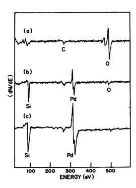
Fig. 4 The Auger eletron Spectrum of the samples; (a) as prepared (b) and (c) during Ar ion sputtering C and O are the main impurities at the surface from (a).
