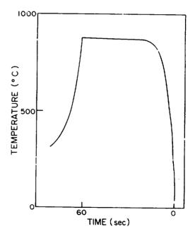
Fig. 2 A typical temperature curve obtained by RTA.
