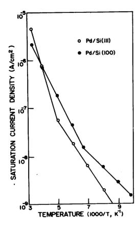
Fig. 8 Temperature dependence of saturation current density for n-type Si(111) and Si(100) at 100 K to 300 K.
