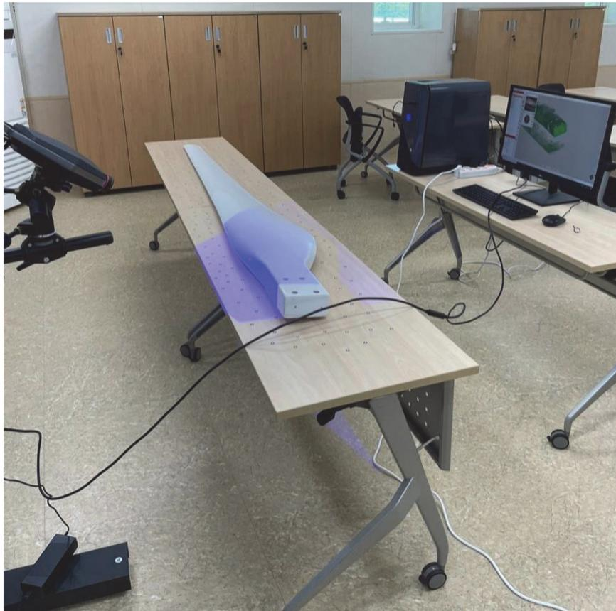
Fig. 25. Picture of 3D scanning process
