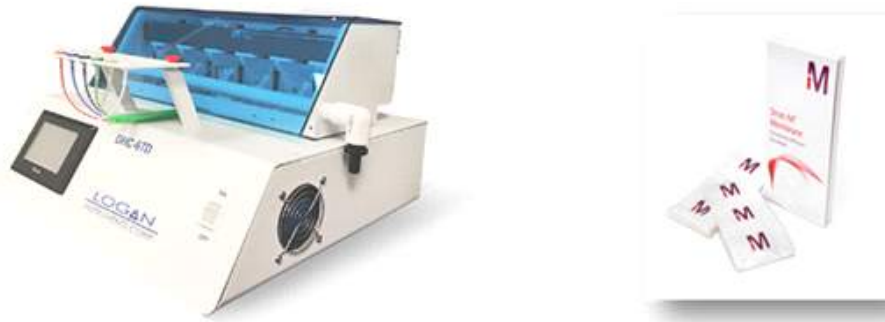
Figure 9. Franz diffusion cell system and Strat-M membrane
