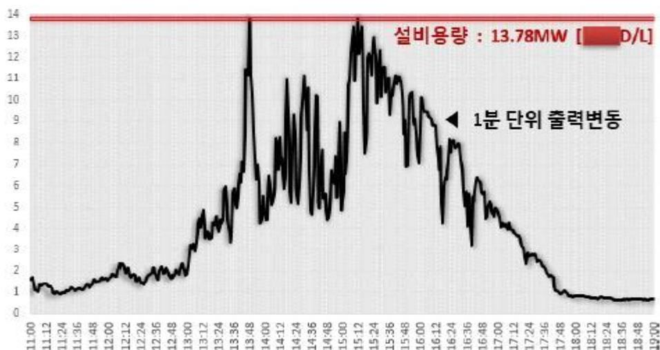
Fig. 4 A PV output by time located in Jeju ('19.03.06 11:00 ~19:00)
