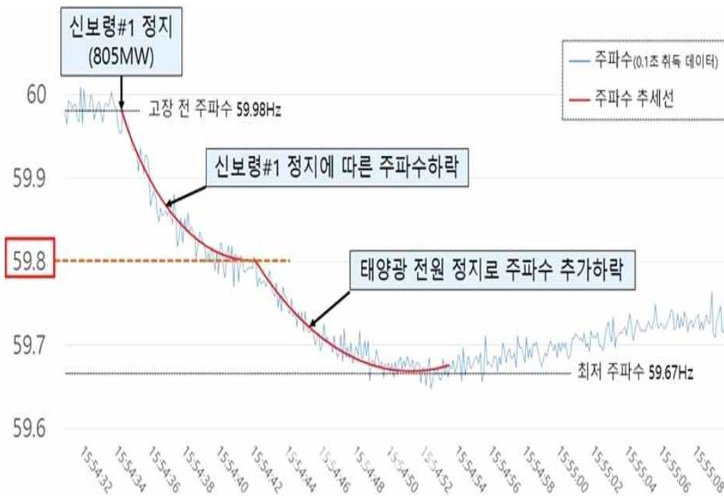
Fig. 16 Frequency according to the trip of Shin-boryeong #1 and PV
