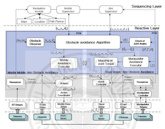
Fig. 5 Overview of integrated navigation system
