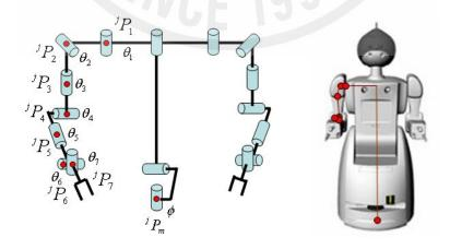
Fig. 19  ${}^{j}P_{i}$  represents the control points on the body.
