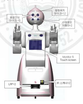
Fig. 7 Robot configuration
