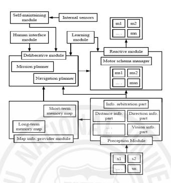
Fig. 3 Control for autonomous robot
