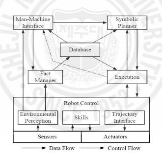
Fig. 2 Hybrid control architecture of care-O-bot
