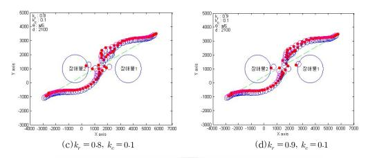
**Fig. 26** Simulations in case of  $k_c = 0.1$ ,  $k_r = 0.6$ , 0.7, 0.8, 0.9
