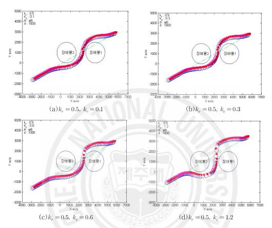
**Fig. 30** Simulations in case of  $k_c = 0.1, 0.3, 0.6, 1.2, k_r = 0.5$
