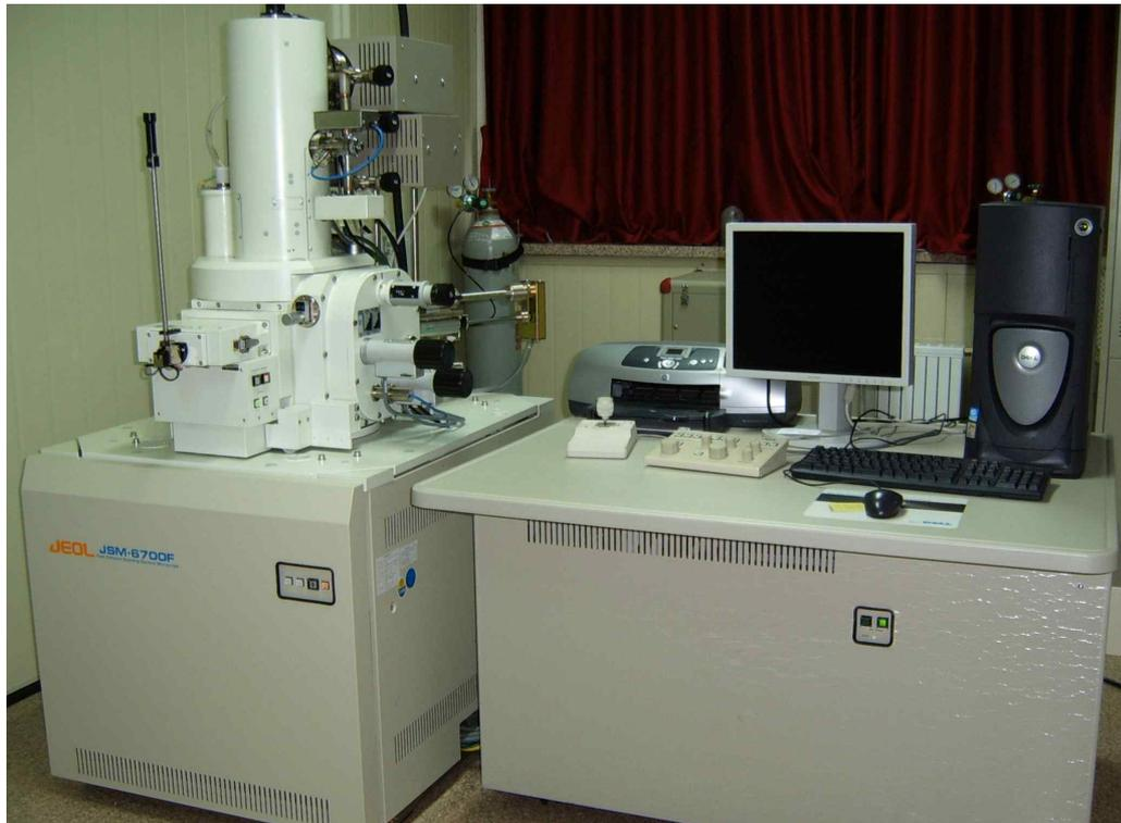
Fig. 5 Field-emission scanning electron microscope.
