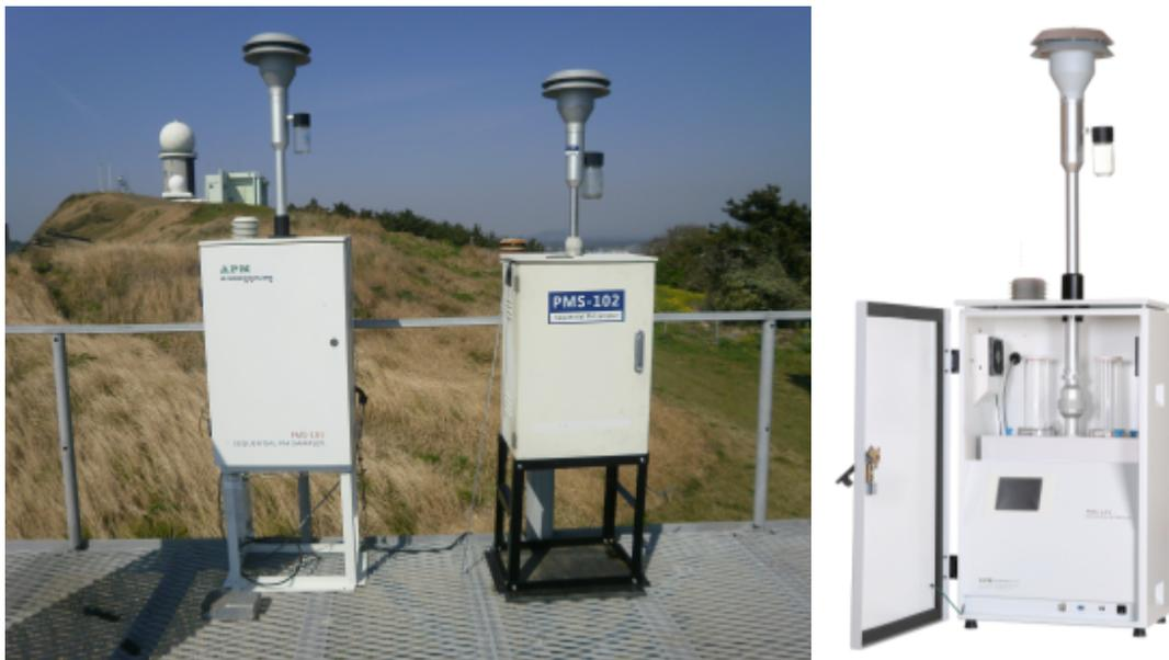
Figure 3. PM<sub>10</sub>/PM<sub>2.5</sub> sequential air sampler (APM Eng., PMS-102, 103, 104).
