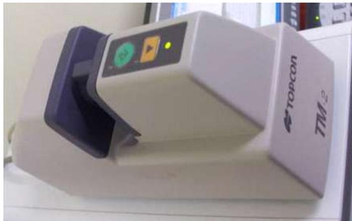
Figure 2. Measuring instrument of luminous transmittance.
