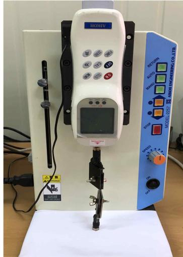
Figure 4. Vertical Motorized Test Stand.
