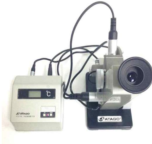
Figure 3. Abbe refractometer.
