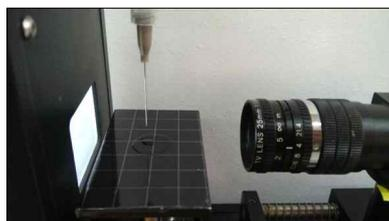
(c) Lens measuring contact angle
