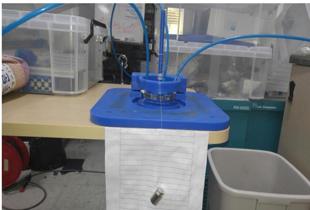
Fig. 18. System for mechanical power calculation in gadolinium generator
