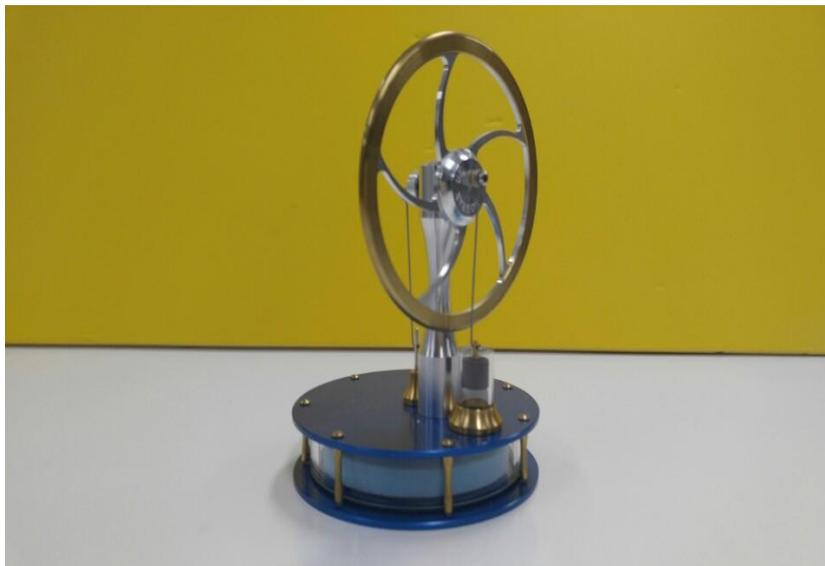
Fig. 9. Photograph of LTD Stirling engine [KS90]
