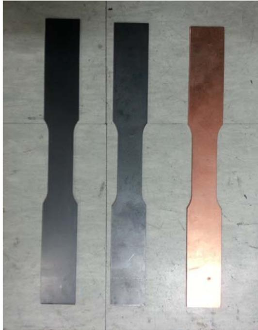
Fig.3 Tensile test specimen
