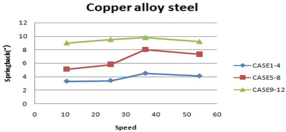
Fig.58 Spring-back of roll forming experiment about copper alloy steel
