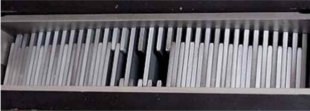
Figure 2. The 64 binary MLC from a Tomotherapy machine. The odd and even leaves are mounted opposite to each other with interfacing. (Dyk J, et al. Tomotherapy: A "Revolution" In Cancer Radiation Therapy. 2013)
