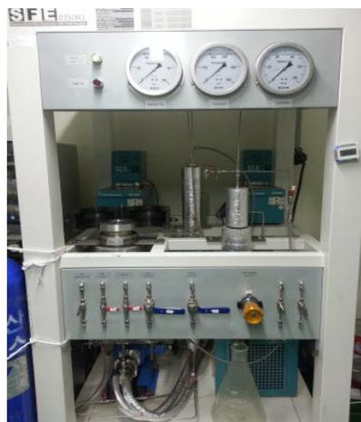
**Figure 1.** Supercritical fluid carbon dioxide extractor used in experiment
