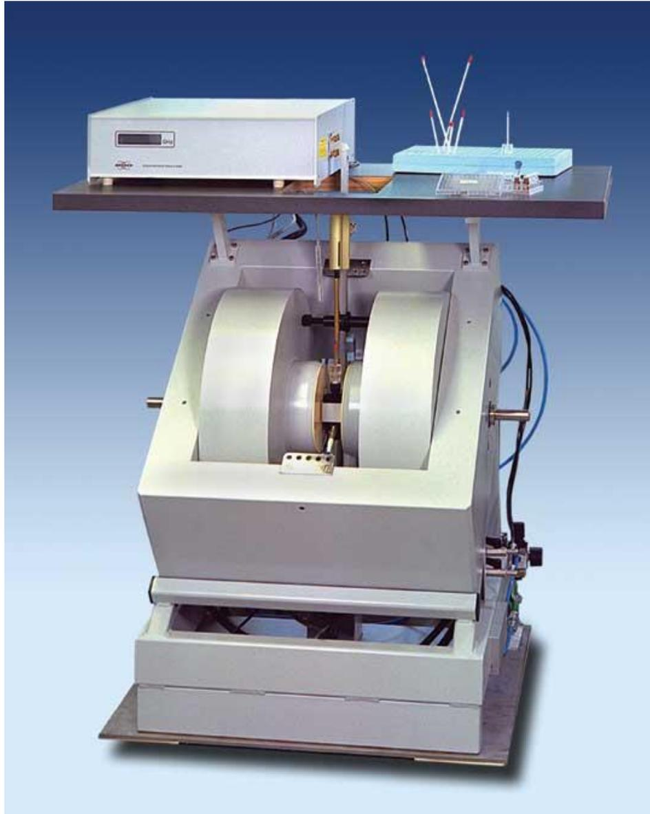
**Fig. 7** Electron Spin Resonance (ESR) spectrophotometer (JES-FA machine, JOEL, Tokyo, Japan)
