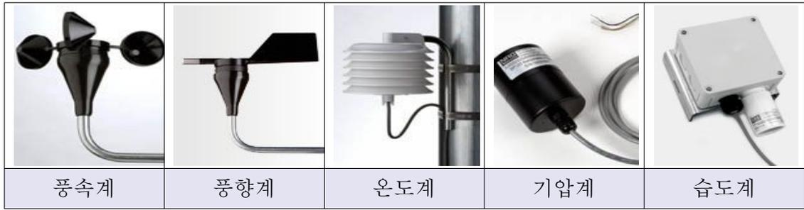
Fig. 17 The pictures of sensor installed on Met. mast..
