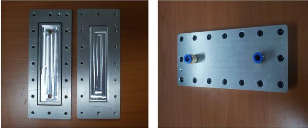
[그림 16] Electrodes with water cooling system
