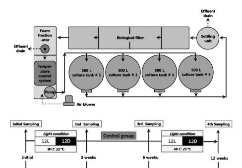
Fig. 2. Recirculating rearing system of schematic diagram and environmental control (photoperiod and water temperature) scheme to sex maturation of *Epinephelus fasciatus*.
