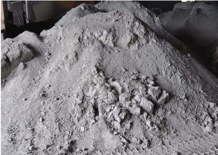
Fig. 7 Stone powder sludge
