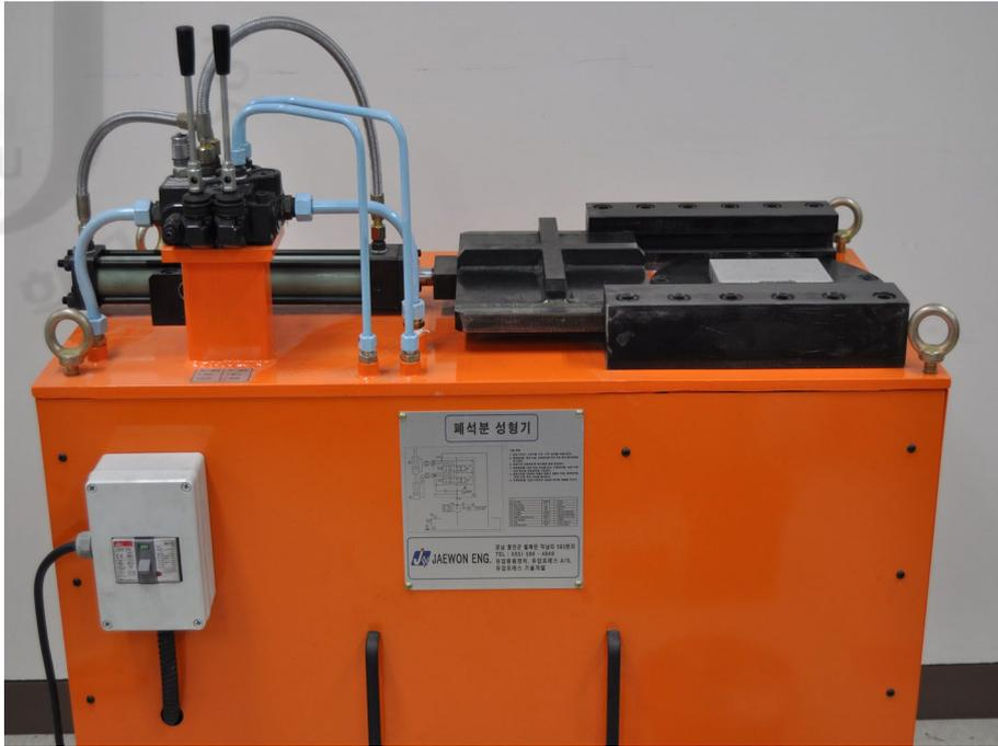
Fig. 17 Waste stone powder molding machine
