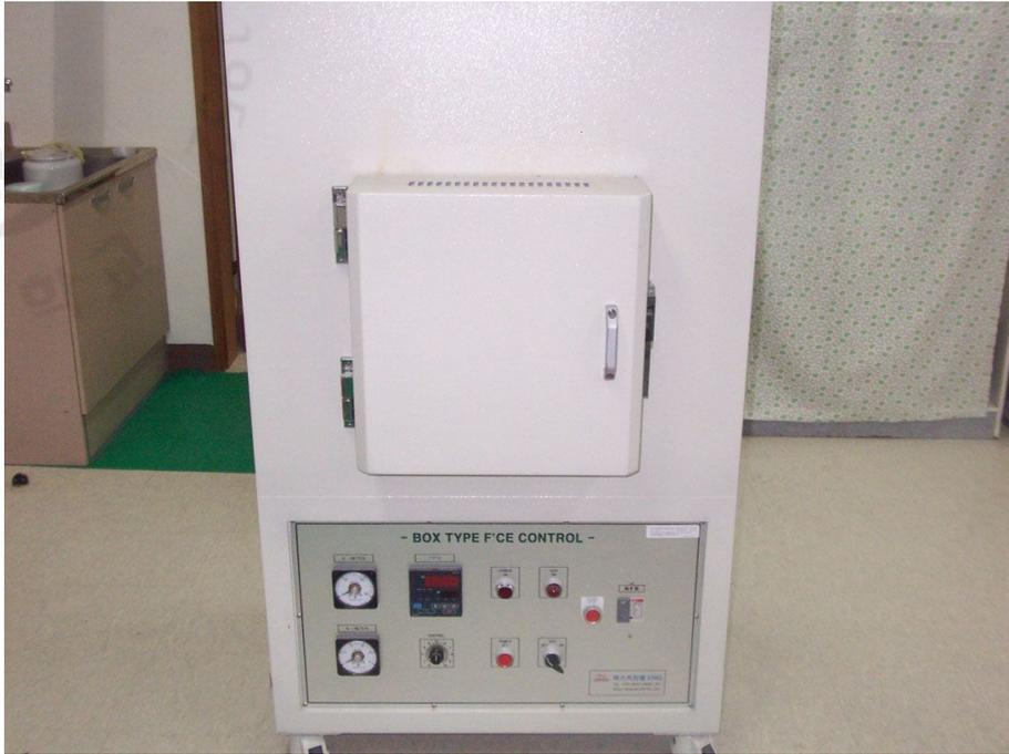
Fig. 20 Outside of electric furnace
