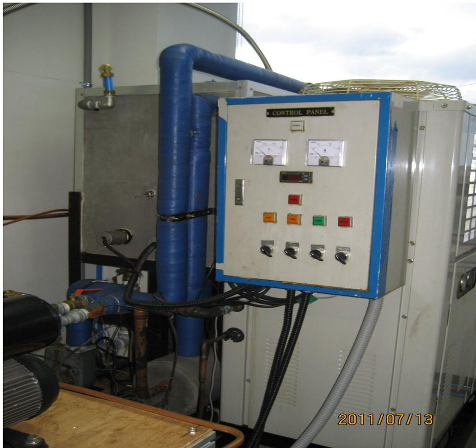
Fig. 12 Chiller for cooling of the outdoor psychrometric chamber
