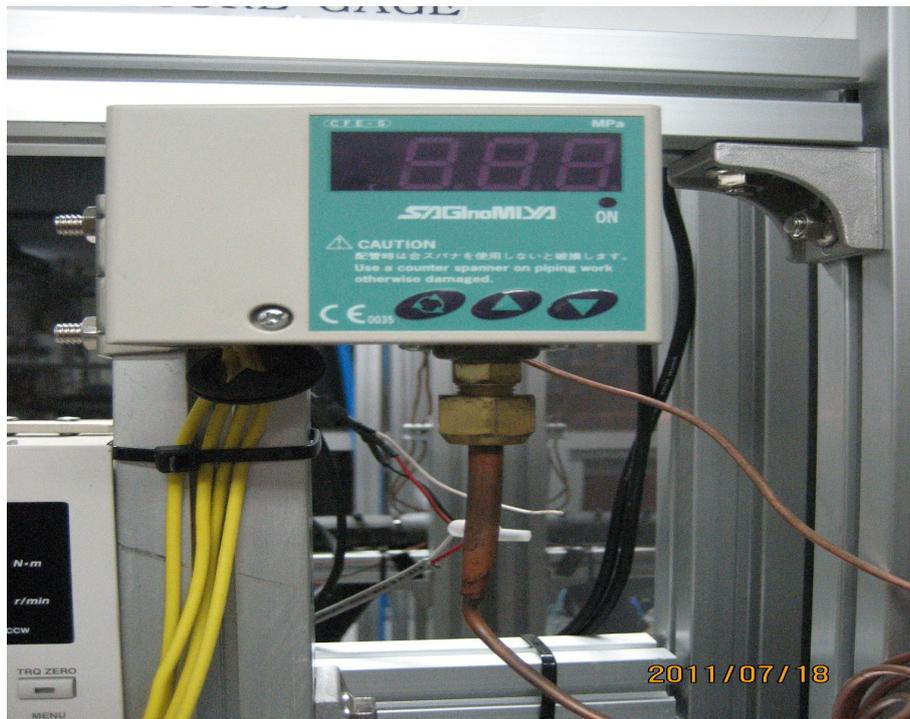
Fig. 18 View of digital low pressure switch
