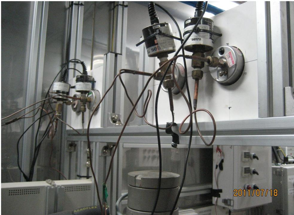
Fig. 23 View of pressure transmitter to measuring cycle pressure of the system
