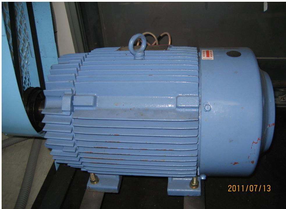
Fig. 16 Picture of 3-phase AC motor with 18.5kW capacity
