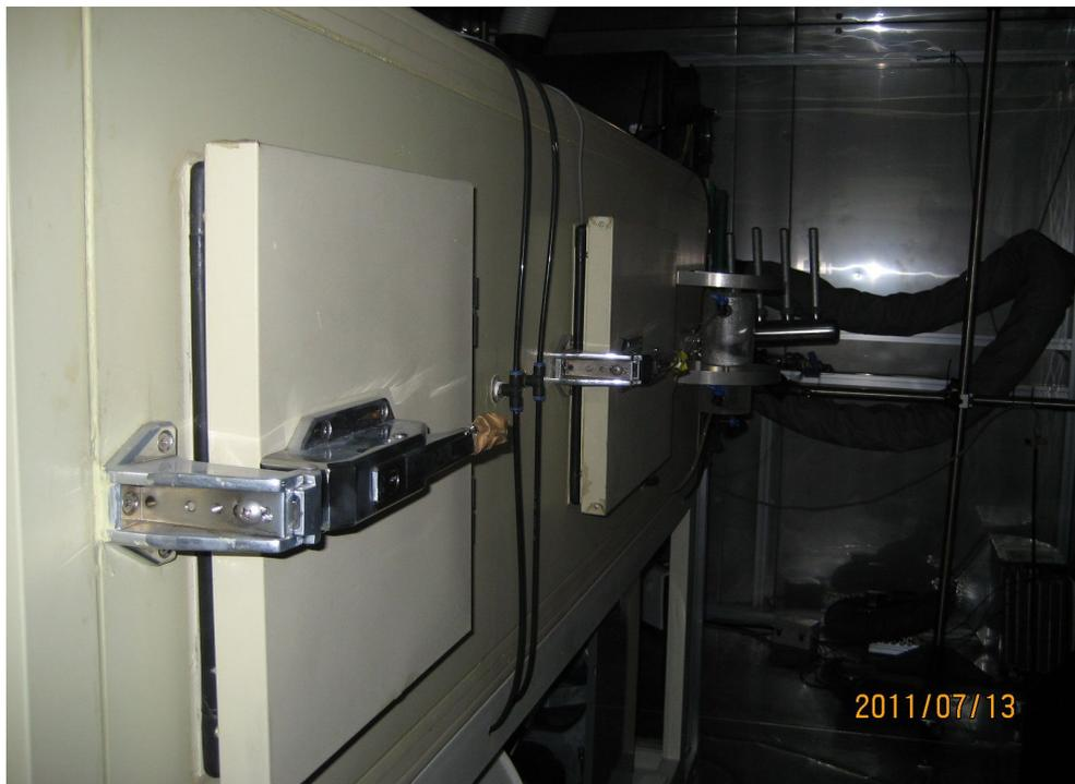
Fig. 14 Cord tester in the indoor chamber for measuring dry and wet bulb temperature and flow rate
