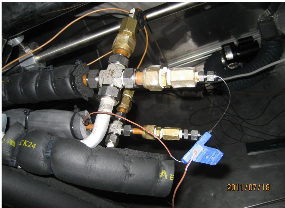
Fig. 20 View of pressure and temperature(Omega 1/16") measuring jig in the refrigerant loop
