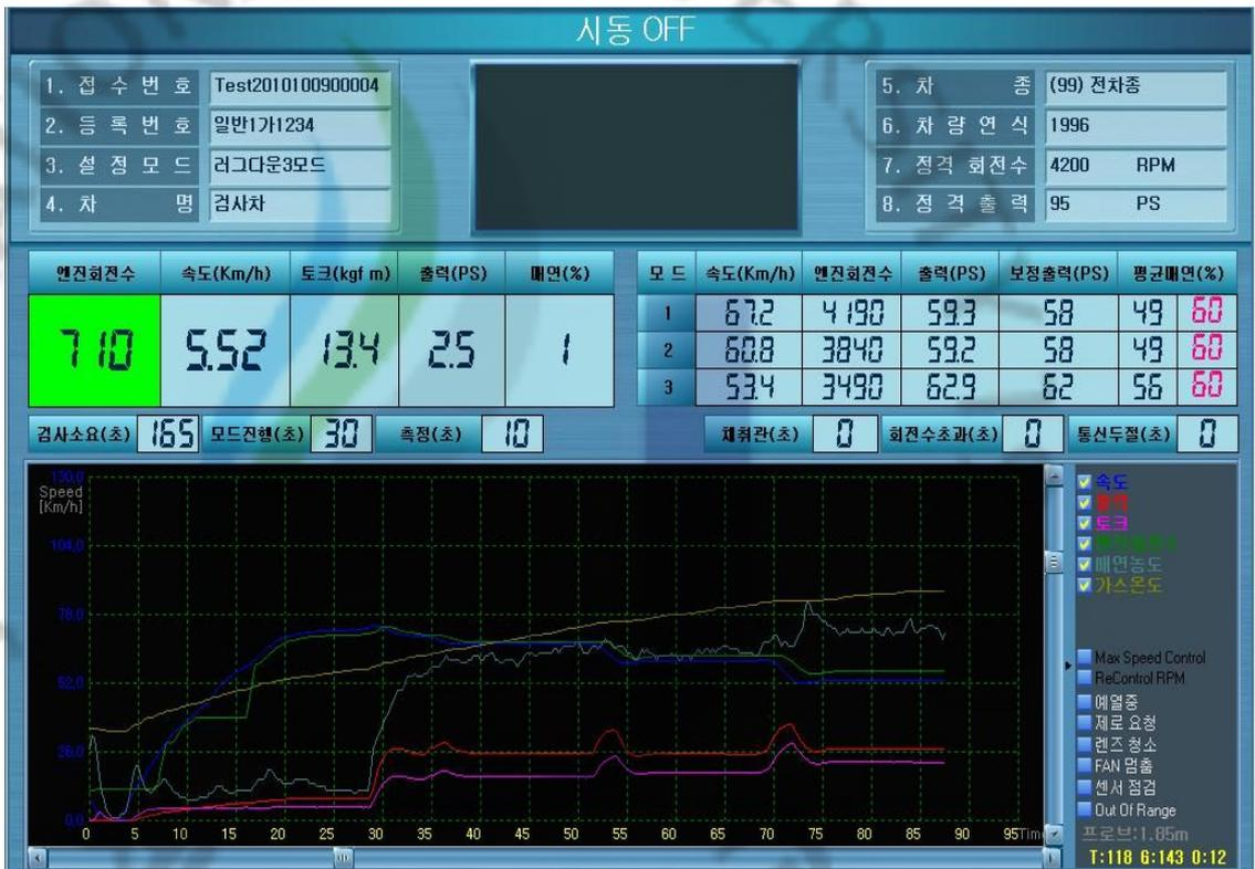
Photo. 3.7 Test result of turn on the air conditioner 4 step(Ball valve close)
