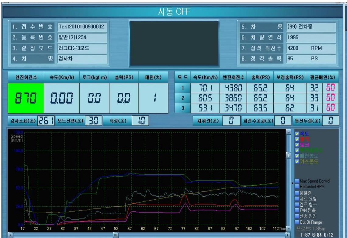
Photo. 3.2 Test result of turn on the air conditioner 1 step(Ball valve open)
