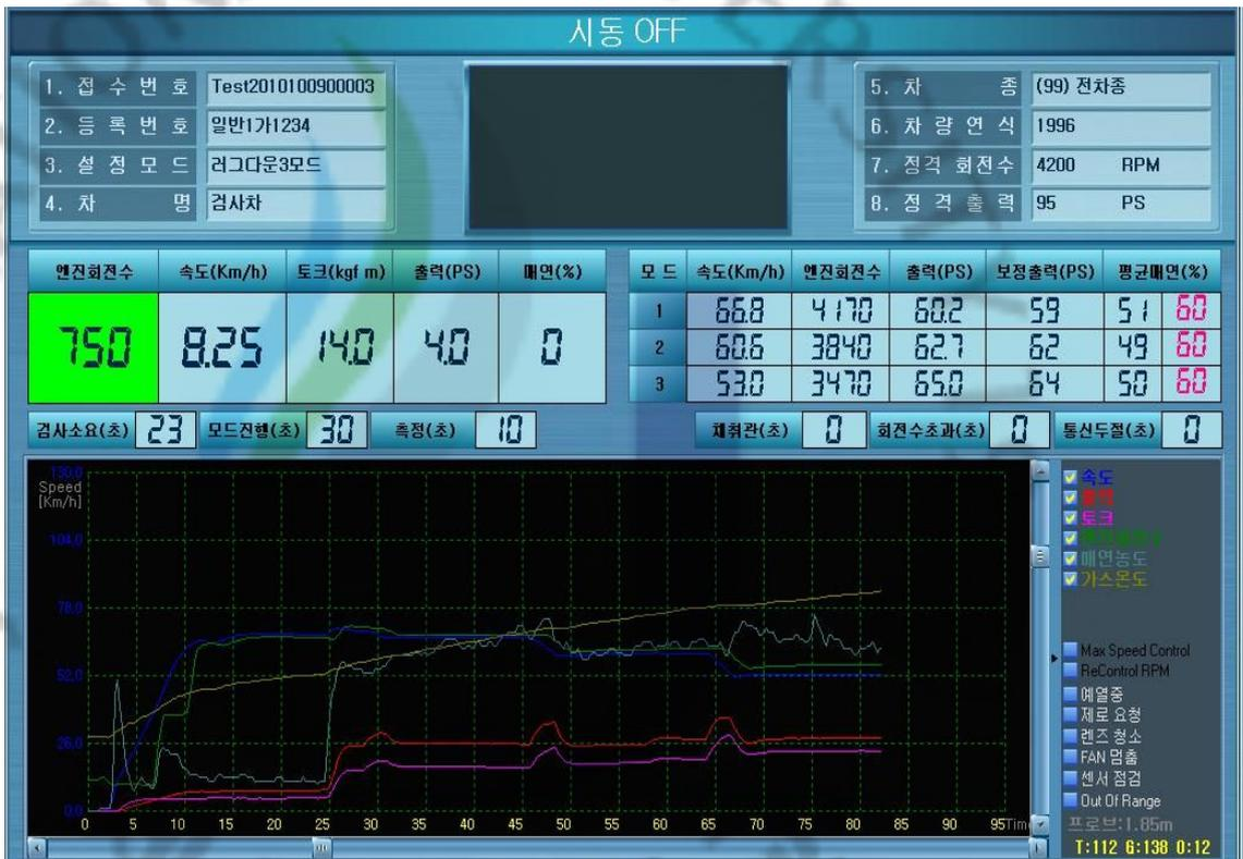
Photo. 3.3 Test result of turn on the air conditioner 2 step(Ball valve close)
