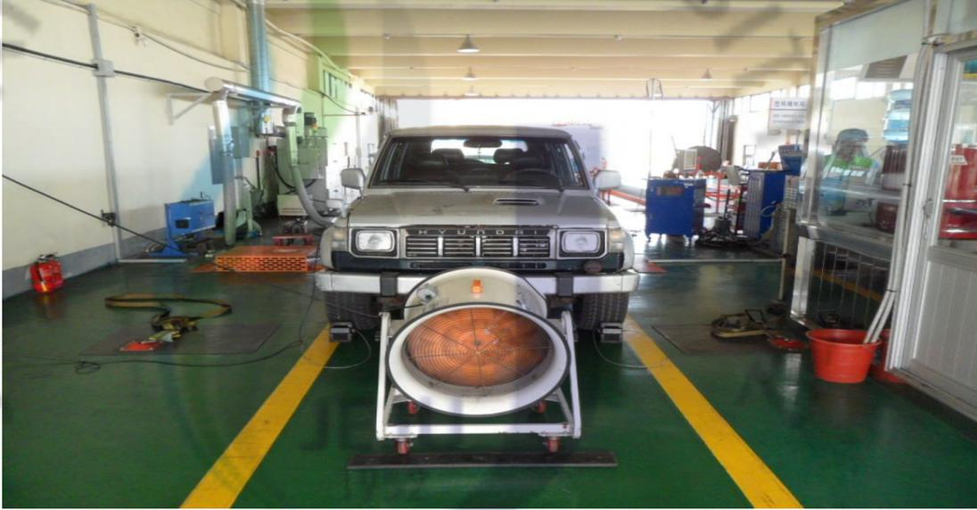
Photo. 2.10 Tested car on chassis dynamometer
