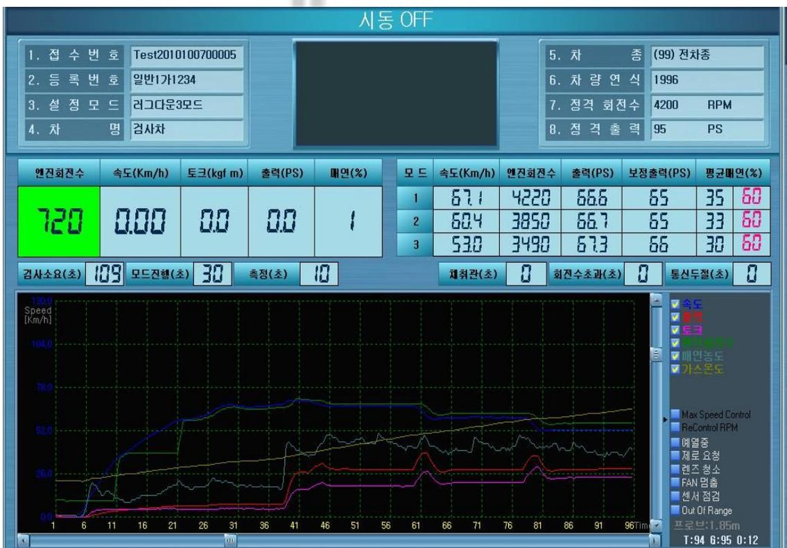
Photo. 3.6 Test result of turn on the air conditioner 3 step(Ball valve open)
