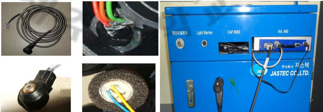
Photo. 2.6 Magnetic type vibration sensor
