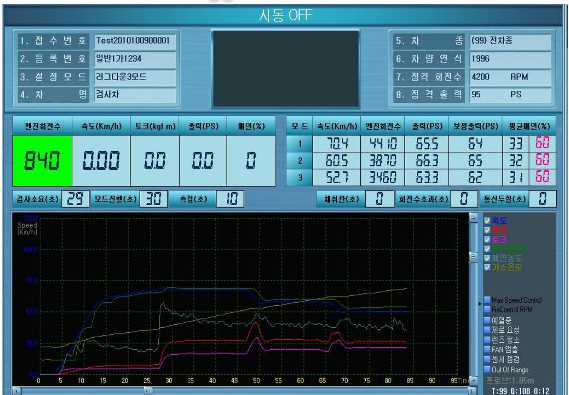
Photo. 3.4 Test result of turn on the air conditioner 2 step(Ball valve open)
