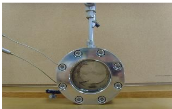
Fig. 21. The measurement reactor of hydrate phase equilibrium and induction time.
