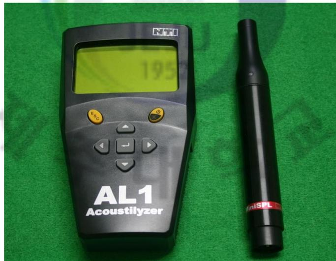
Fig. 27. Acoustic analyzer for measuring characteristics of acoustic waves
