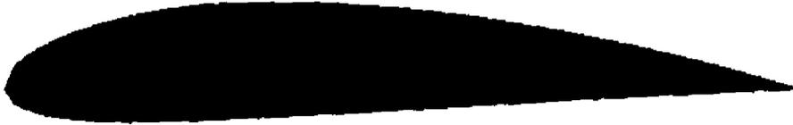
Fig. 2-6 Section shape of NACA 4415
