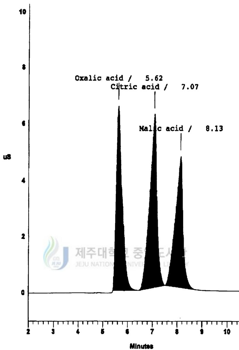
Fig. 1. Bio-LC chromatogram of standard organic acid mixture.
