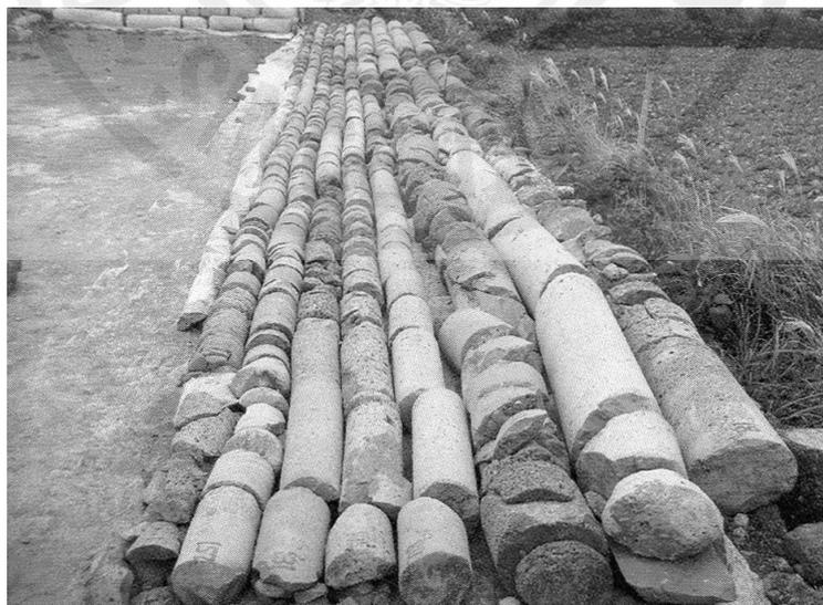
Fig. 3.1 Photograph of collected cores
