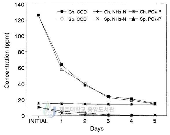
Fig. 13. Change in the quality of exhausted water after incubation with one of two microbes (*Chlorella vulgaris* and *Spirulina platensis*) and PSB. Either *C. vulgaris* or *S. platensis* was inoculated first and then the PSB was sequencially added with one-day interval. Ch: *Chlorella vugalis*, Sp: *Spirulina platensis*.
