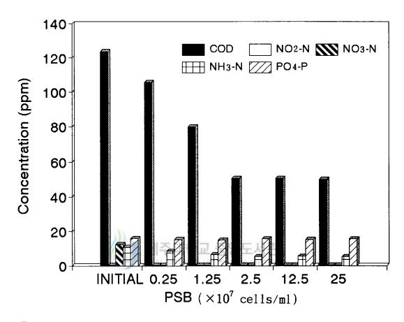
Fig. 11. Change in the quality of exhausted water after the two-day incubation with the PSB. Inoculations were conducted once a day and were begun with five different densities.
