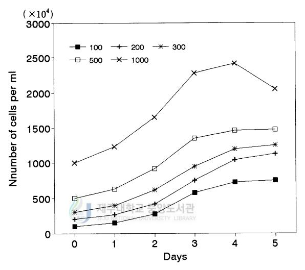
Fig. 4. The growth curve of *Chlorella vulgaris* in exhausted water, depending on its incubated period and inoculated conentration (unit:  $\times 10^4$  cells/ml).
