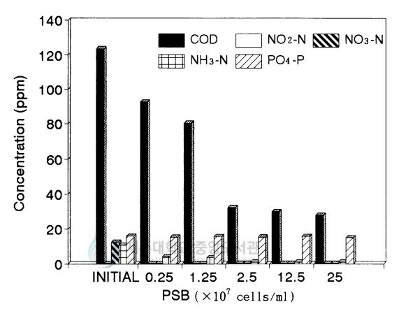
Fig. 12. Change in the quality of exhausted water after the three-day incubation with the PSB. Inoculations were conducted once a day for three days and were begun with five different densities.
