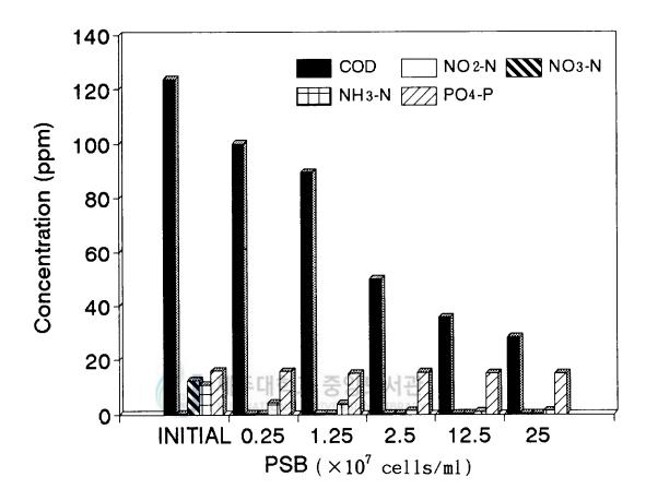
Fig. 10. Change in the quality of exhausted water one day after the single inoculation of the PSB with five different densities.
