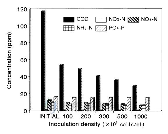
Fig. 9. Change in the quality of exhausted water five days after the single inoculation of *Spirulina platensis* with five different densities.
