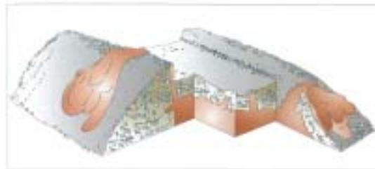
Fig. 4.3 Sectional diagram of aa lava flows
