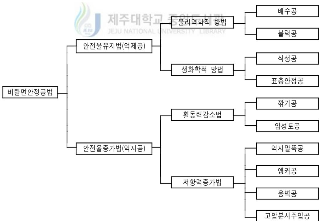
Fig. 5.1 Classification of slope stabilization methods
