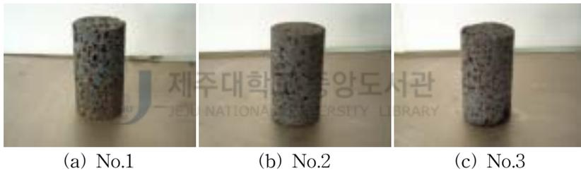
Fig. 4.6 Specimen before uniaxial compression test
