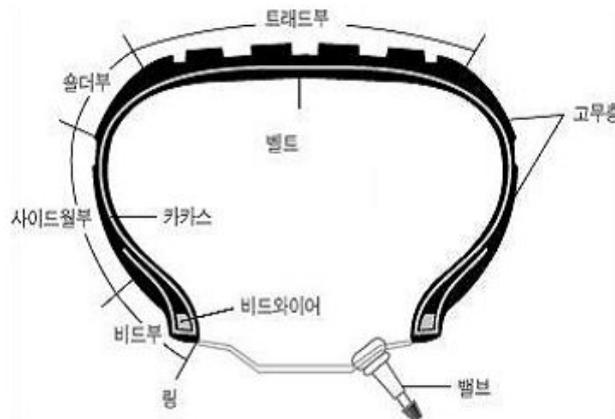
Fig. 3.1 General structure of the tire
