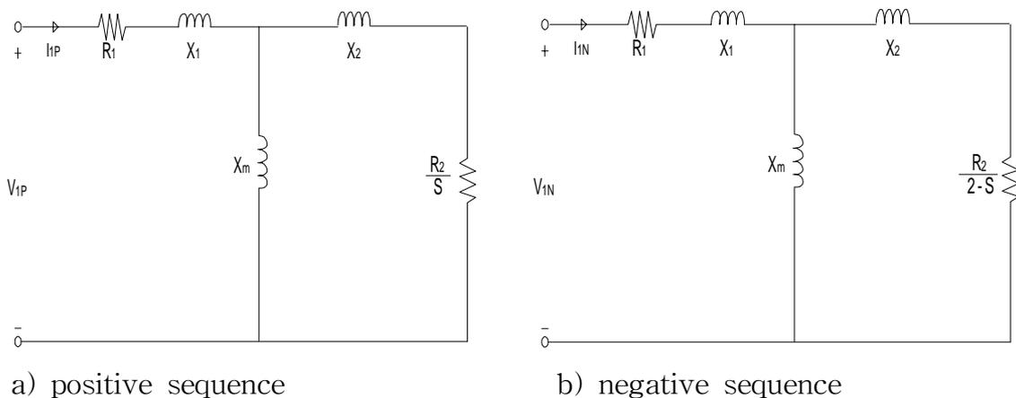
Fig.1 Equivalent circuits of model machine
