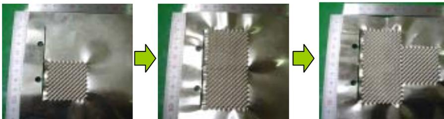
Fig. 51 Embossing shape of inner structure
