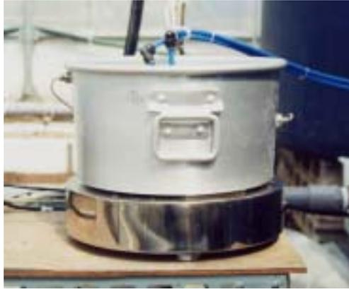
Fig. 10. Nutrient solution weight measuring equipment.
