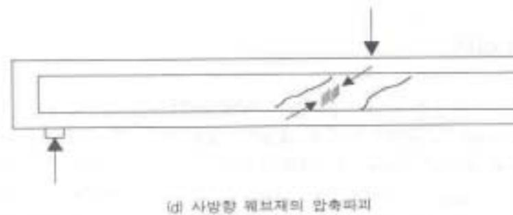
Fig. 3 Shear failure modes
