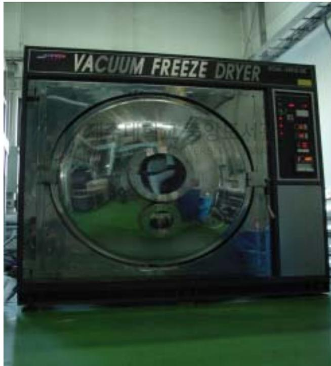
Fig. 2. Lyophilization through vacuum freeze dryer.
