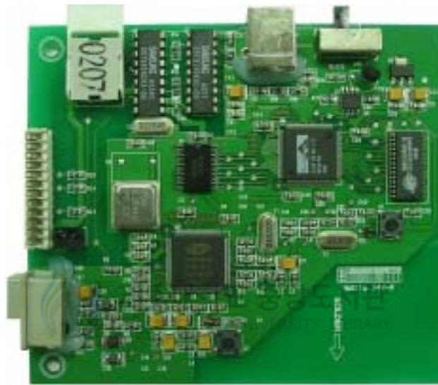
Fig. 17. DSP board for voice processing
