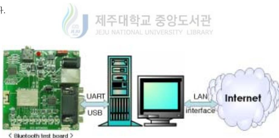
Fig. 20. Bluetooth LAN access point configuration based on PC
