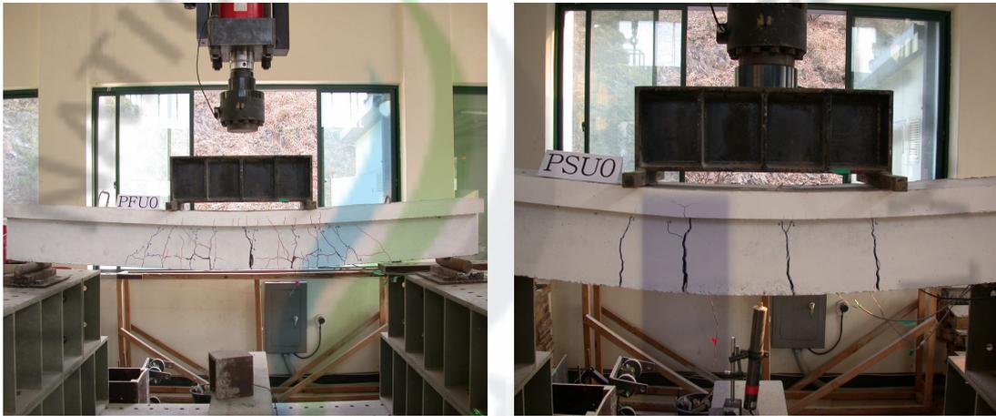
Fig. 5.3 Real view of static test (PFU0(left) and PSU0(right))
