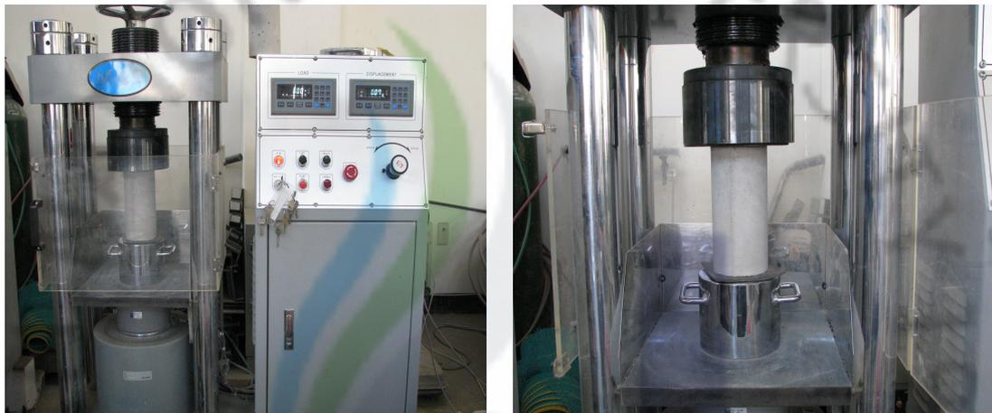
**Fig. 3.5 Compressive strength test**
