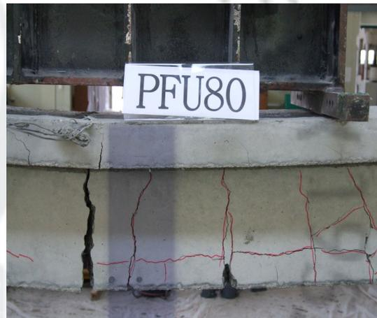
Fig. 5.21 Crack details after failure
