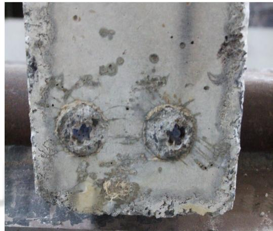
Fig. 5.27 Debonding of concrete and tendon
