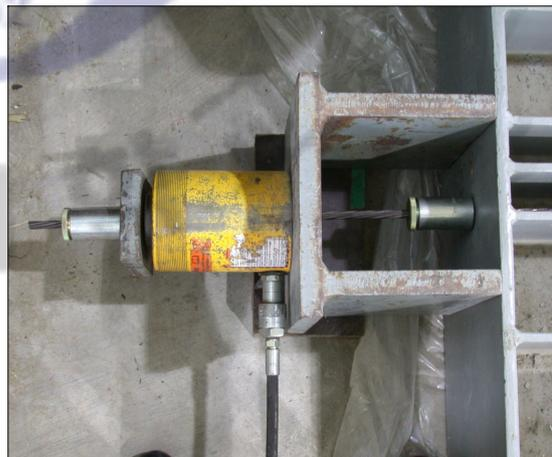
Fig. 3.13 Jacking of FRP tendon(left) and Steel tendon(right)
