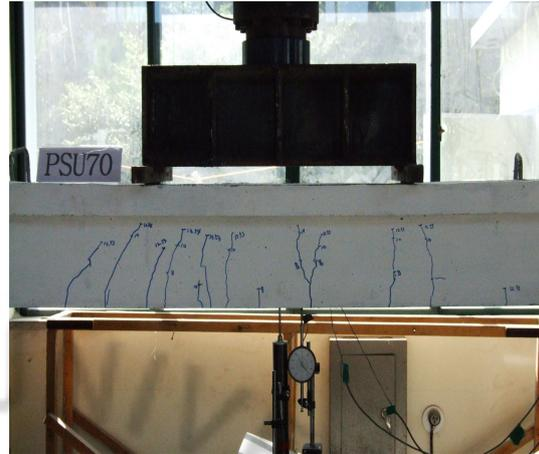
Fig. 5.37 Crack propagation
