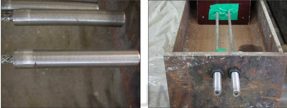
Fig. 3.9 Compression type anchorage
