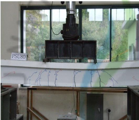
Fig. 5.44 Crack view after 10<sup>3</sup> cycle
