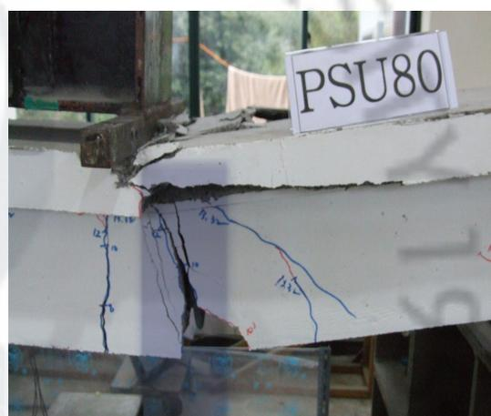
Fig. 5.45 Failure view of 2,300 cycle
