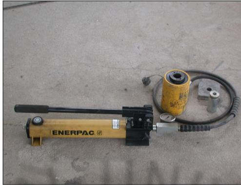
Fig. 3.11 Hydraulic jack for tensioning
