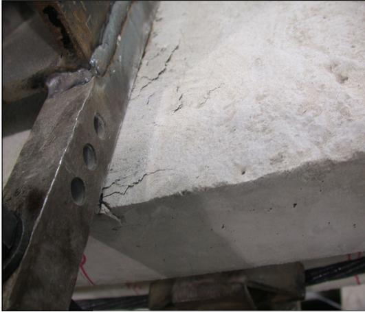
(a) Cracks at top flange
