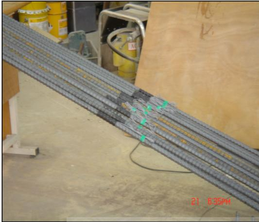
(a) Strain gages on reinforcing bars
