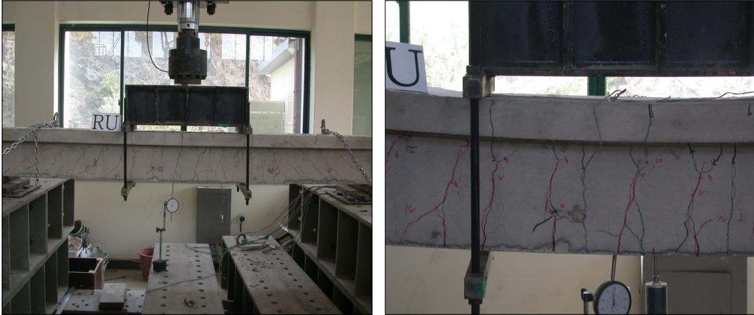
(c) Cracks after concrete compression (d) Crack details after failure failure
