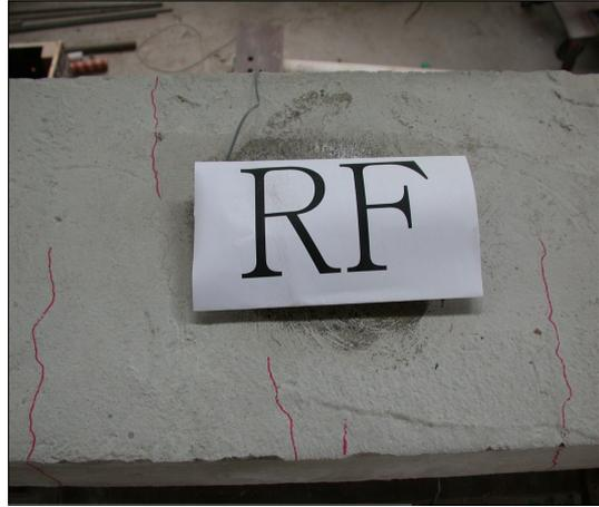
(b) Cracks at top flange
