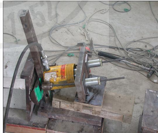
Fig. 3.7 Jacking of steel tendon
