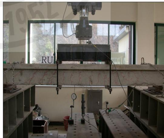
(b) Crack propagation
