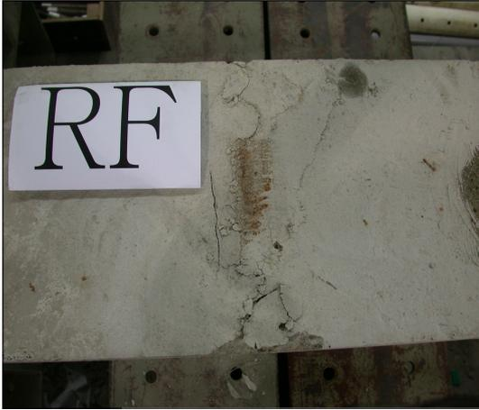
(a) Cracks at top flange
