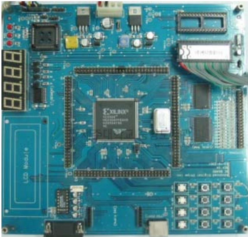
Fig. 27. Test board for bluetooth core design
