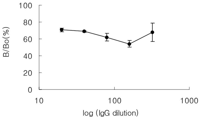
Figure 3. Determination of the optimal dilutes of anti-SMZ antibody. Each well was coated with varying dilutions of immunoaffinity purified IgG. SMZ ( $0.1\mu\text{g/g}$ ) and SMZ-HRP (1:200) in PBS-tween 20 solution were added. B/Bo (%) were calculated according to the following formula:  $\text{B/Bo (\%)} = (\text{absorbance at } 0.1\mu\text{g/g of SMZ} / \text{absorbance at } 0\mu\text{g/g of SMZ}) \times 100$ . The error bar indicates standard deviation.
