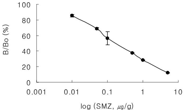
Figure 4. Standard curve of SMZ obtained by the direct competitive ELISA. Each well was coated with anti-SMZ IgG (1:160). SMZ standard and SMZ-HRP conjugate (1:200) solution were reacted. B: Absorbance of SMZ standard, Bo: Absorbance of blank solution.
