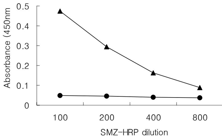
Figure 2. Effect of detergent (Tween 20) on nonspecific binding SMZ-HRP to plate well. The well was coated with affinity purified antibody, blocked with ovalbumin, SMZ-HRP reagent, substrate and stop solution, were added sequentially. SMZ-HRP diluted in PBS containing Tween 20 (●). SMZ-HRP diluted in PBS (▲).
