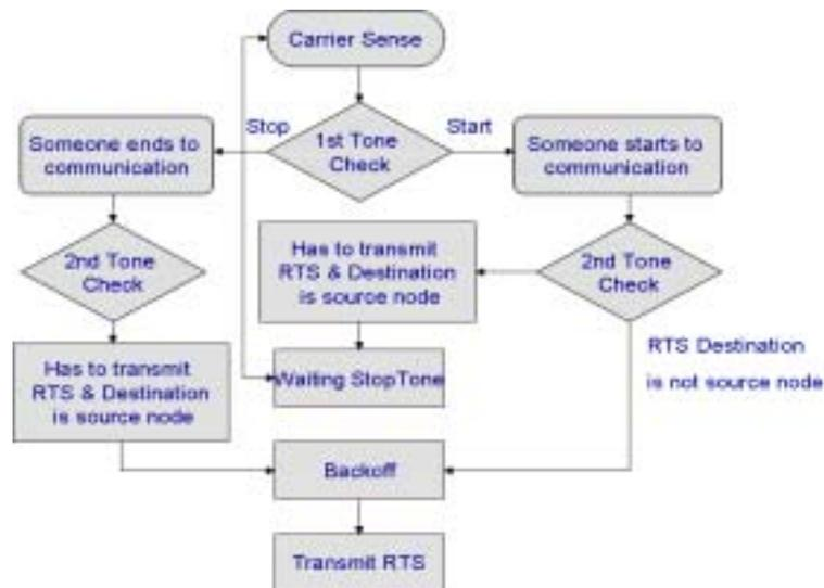
Fig. 15. The procedure of the proposed MAC protocol with dual tone
