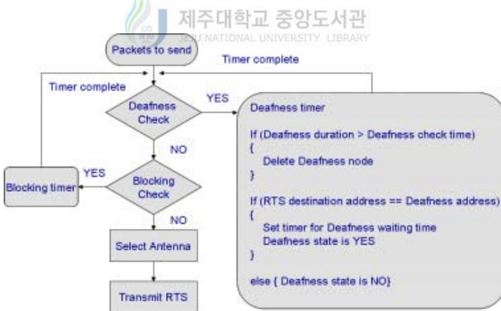
Fig. 12. The procedure of a RTS frame transmission
